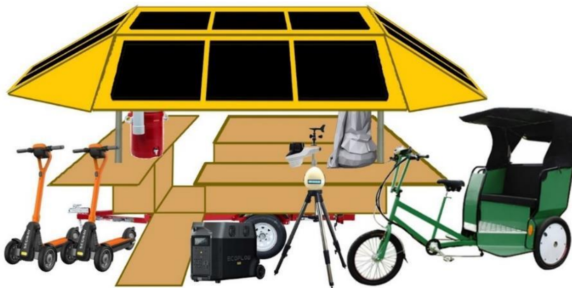
Figure 28: Solar Docking/Charging Station for Electric Micromobility
