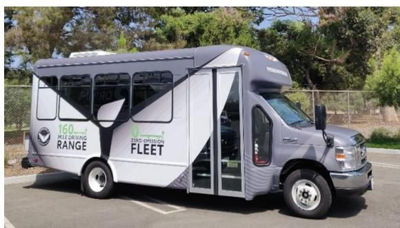
As an EV pioneer, we delivered their first commercial EV in 2014. We develop and integrate their proprietary electric drivetrain into the Ford E-Series Chassis. The range of configurations vary from shuttle buses, Type A school buses, utility trucks, service trucks, to flatbed trucks, walk-in vans, and cargo trucks. Since their inception, we have been
